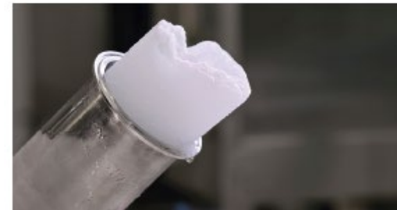
Figure 2. showcases how the ice slurry is formed into a solid know as an "ice-pig" once pumped into the pipeline.
